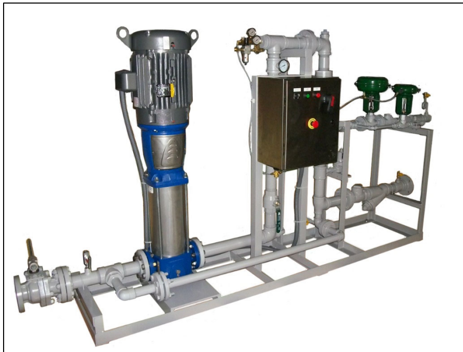
Figure 1. Pick's approach was to combine two of its primary design strategies into a single system: a constant-flow DSI heater, along with a variable-frequency drive (VFD) on a downstream boost pump. Source: Pick Heaters Inc.
